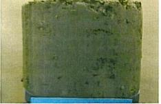
Note: A B-value of 0.97 was achieved for the undisturbed specimen. Permeation measurements were made with a mercury Utube. The effective confining pressure was 5 psi per test request.
