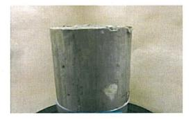
Note: A B-value of 0.95 was achieved for the undisturbed specimen. Permeation measurements were made with a mercury U-tube. The effective confining pressure was 5 psi per test request.
