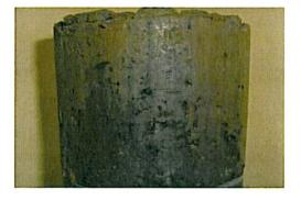
Note: A B-value of 0.97 was achieved for the undisturbed specimen. Permeation measurements were made with a mercury Utube. The effective confining pressure was 5 psi per test request.
